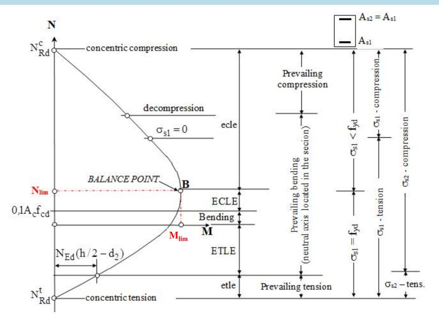
$N_{Rd}^{c} = A_{c}f_{cd} + (A_{s1}+A_{s2})f_{yd}$  - resisting compressive force
