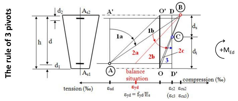
Increasing M<sub>Ed</sub>: - section is rotated around pivot C until reaches the decompression state (line OB)
