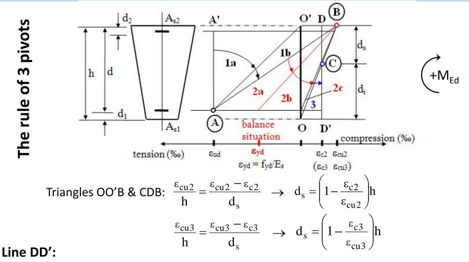
$$\begin{split} -N_{Ed} \& M_{Ed} &= 0: \text{-section in concentric compression} \\ &- \text{crushing of compressed concrete } (\epsilon_c = \epsilon_{c2} \text{ or } \epsilon_c = \epsilon_{c3}) \\ &- \text{reinforcement yields: } \epsilon_{yd} = f_{yd}/E_s (\text{slide 18}) < \epsilon_c (\epsilon_{c2} = 2\%; \epsilon_{c3} = 1,75\%) \end{split}$$
